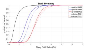
Figure 6. Fragility curves for all CFS walls with steel sheet sheathing.
