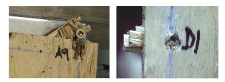
*Figure 2. Examples for failure of walls with WSP sheathing (corresponding to DS3):* (a) *Sheathing tear-out at corners; (b) Wood Bearing Failure (image source:* [3])
