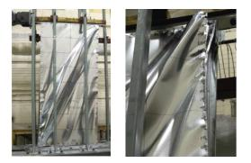
*Figure 5. DS3 example for walls with steel sheet sheathing (a) buckling of steel sheet; (b) Twisting of stud (image:* [6])
