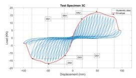
Figure 1. Example of damage states for a test specimen; test data from Boudreault (2005).
