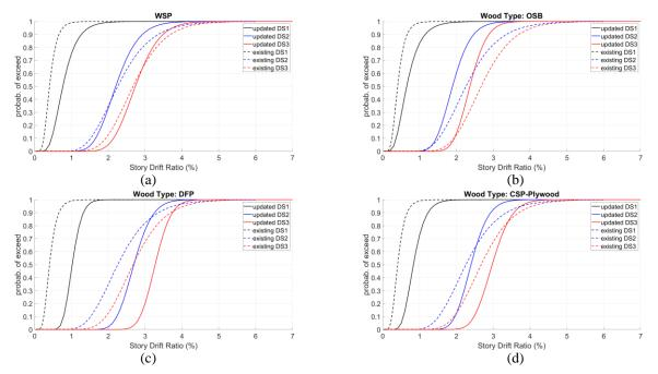
Figure 4. Fragility curves for CFS walls with WSP sheathing: (a) all; (b) OSB; (c) DFP; (d) CSP or Plywood. Table 2. Parameters of fragility curves for CFS walls with WSP sheathing. Demand parameter: Story Drift Ratio (%)
